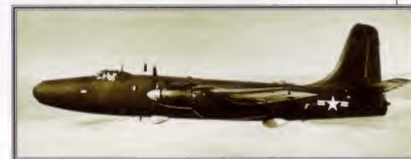
▲ Designed for speed and range Like the Consolidated PB4Y before it, the P4M used a long, thin wing to provide fuel capacity and long range. The jet engines, while providing more speed, actually compromised range performance.
